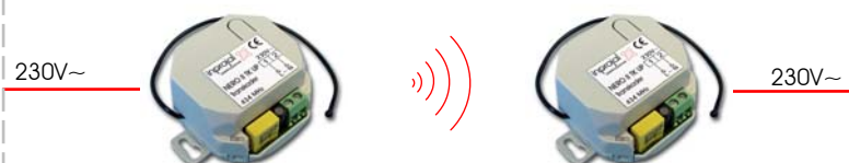
Example 5: Bridging a galvanic isolation (Radio bridging)
